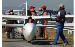
Glide Ratio of gliders is from 30 of trainer to 60 of racer, which means it has a performance of 30km to 60km of distance to fly if the glider is cruising at 1000m height. And the gliders are employed with the ultimate state of arts technologies. Glider sports is a combination art of using these performance and the knowledge on the power of natural
